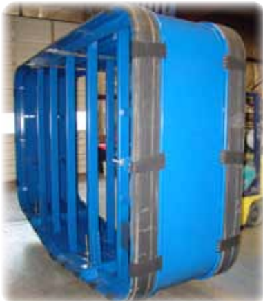
Joint Tester built to vacuum test 120" V-Shaped concrete pipe.
