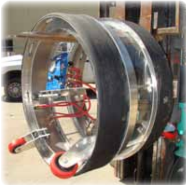
Custom Vacuum Joint Tester. Uses vacuum to test welds on steel, mortar-lined pipe.
