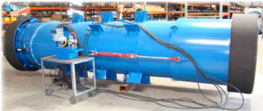
66" Hydraulically Actuated Telescopic Flow Diverters used to dry up a structure in Denver, CO. Diverters are steered into place remotely with included hydraulic control panel.
